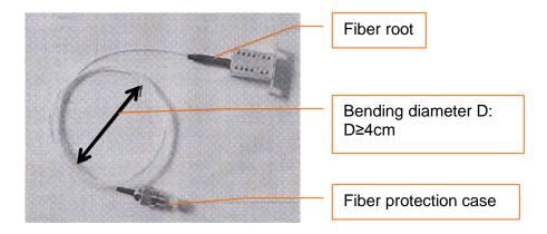
Make sure that the module and the fiber are in the same plane.
